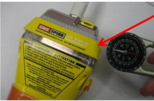
A Compass provides simple detection on bracket magnet.
