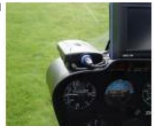
Uses aircraft power supply no battery backup
