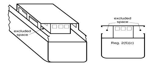
R.2(5)-2 In the case of a ro-ro ship, for example, where the space at the end of an erection is fitted with means for securing cargo, the space should be included in V in accordance with the first condition of regulation 2(5).
