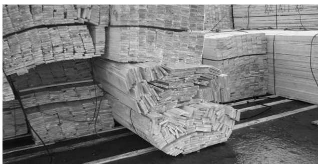
Figure 6.2. Example of poor rigidity
