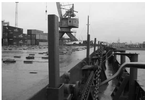
Figure 6.7. Example of uprights for bottom blocking
