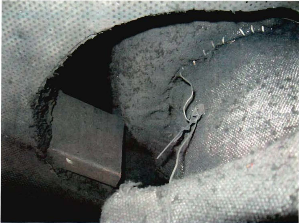
Steamer DELTA QUEEN CO2 Protected Generator Enclosures not Fume-tight -- 5/2008
