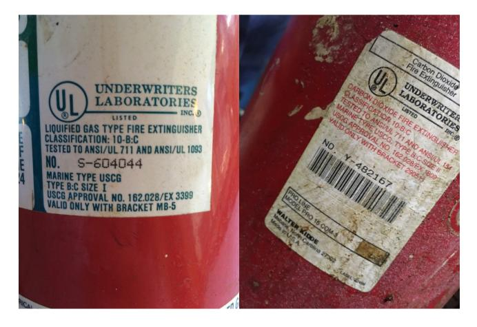
According to the new carriage requirements, a minimum required rating of 20-B:C is necessary in the pilothouse. Neither the 5lb. liquefied gas extinguisher or the 15 lb. or 20 lb. carbon dioxide extinguisher meets the updated requirements. These extinguishers are rated as a 10-B:C under this classification but have been the most appropriate for use in the pilothouses of vessels for many years.
