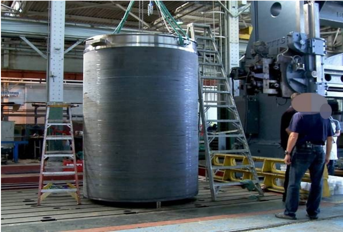
Figure 89: Aft titanium segment being placed on the first TITAN carbon fiber hull in July of 2017. Source: OceanGate Expeditions.
