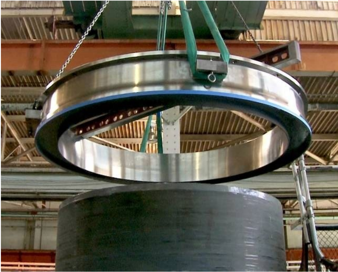
Figure 88: Adhesive applied to carbon Fiber Hull and “c” channel of forward segment in July of 2017. Source: OceanGate Expeditions.
