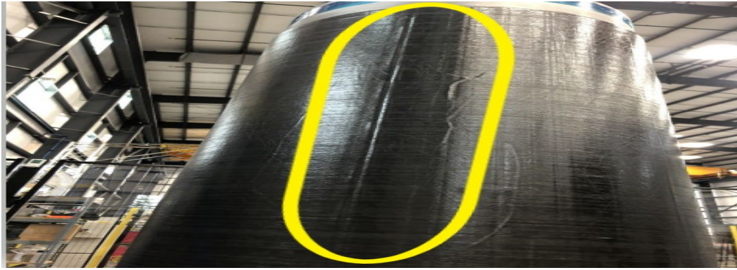
Figure 139: Wrinkle in the one-third scale hull model for Final TITAN hull (yellow circle added by MBI). Source: OceanGate Expeditions.
