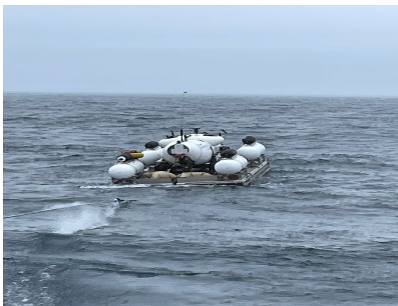
Figure 240: TITAN being towed by POLAR PRINCE on May 25, 2024, with missing tail cone due to the May 24 th incident, heading to Witless Bay, Newfoundland for a damage assessment. Source: Former mission specialist.
