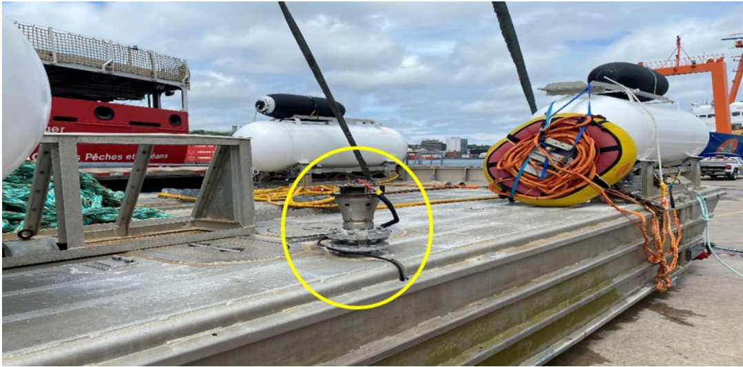
Figure 112: The LARS ballasting valve is pictured within the yellow circle added by MBI. The photograph was taken by the MBI in St. John's, Newfoundland post-casualty on June 25, 2023. Source: USCG.
