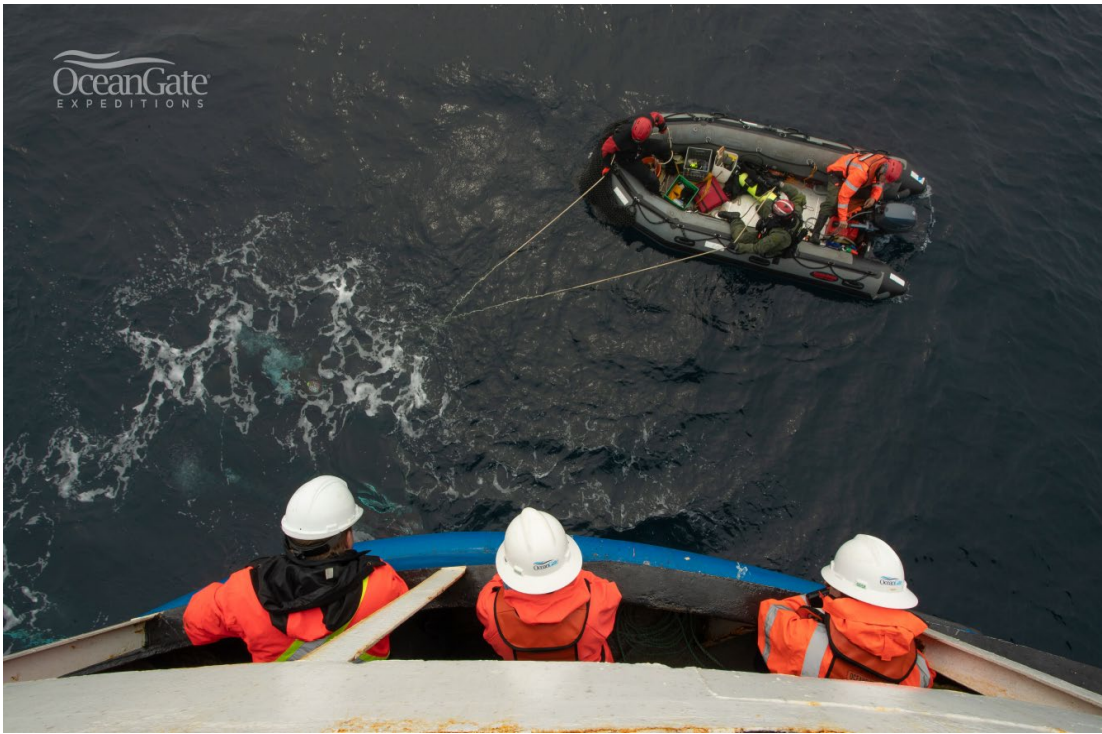
Figure 244: Overhead view from POLAR PRINCE of divers attempting to remove a towline that had fouled POLAR PRINCE's propeller on June 7, 2023. Source: OceanGate Expeditions.
