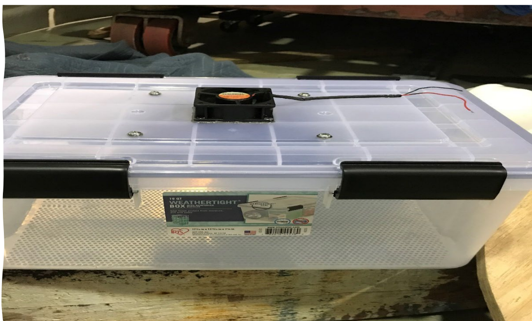
Figure 178: TITAN's "homemade" CO 2 scrubber. Source: Former Director of Marine Operations.
