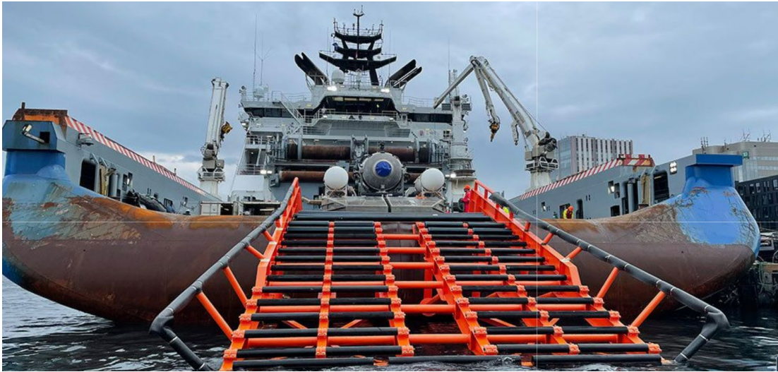
Figure 196: TITAN launch and recovery ramp deployed from the stern of the HORIZON ARCTIC on June 29, 2021. The HORIZON ARCTIC served as TITAN's support vessel during the 2021 and 2022 TITANIC Expeditions. Source: OceanGate.
