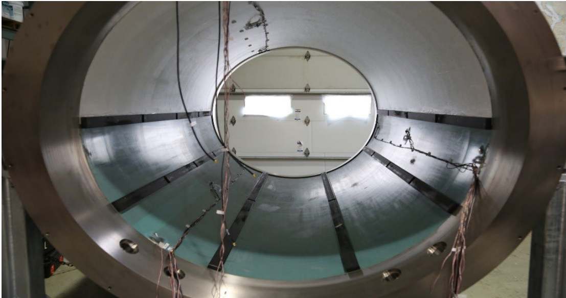
Figure 121: Image of TITAN's interior hull shows the acoustic emission and strain gauge instrumentation locations. Source: Former OceanGate Director of Engineering Report.
