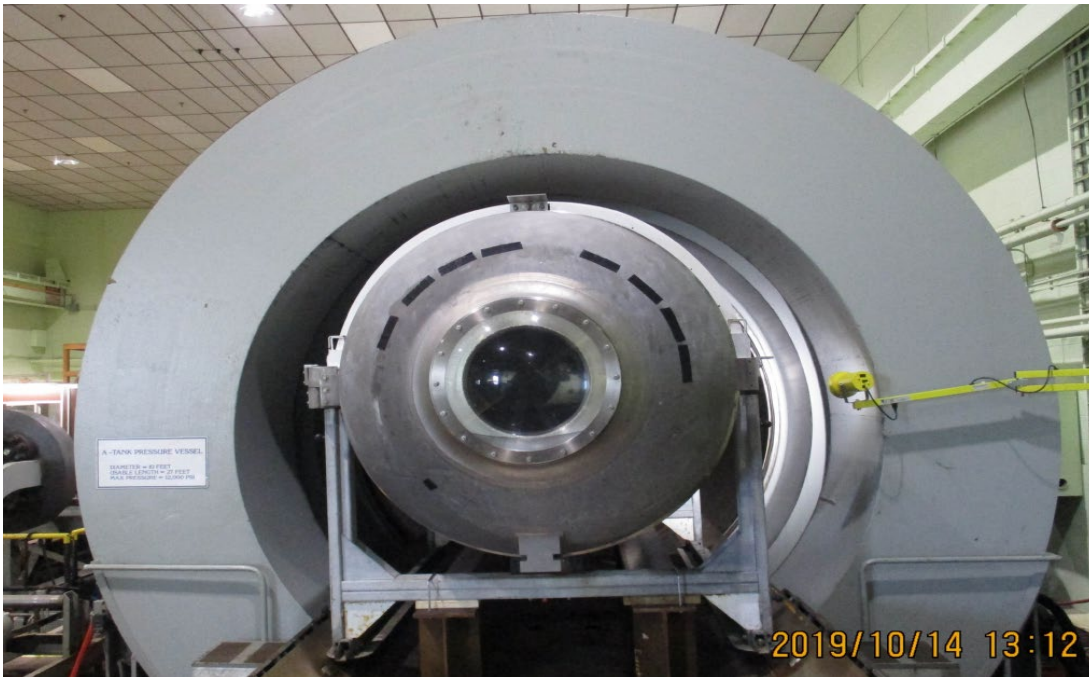
Figure 134: First TITAN hull inside Deep Ocean Test Facility chamber on October 14, 2019. Source: OceanGate.
