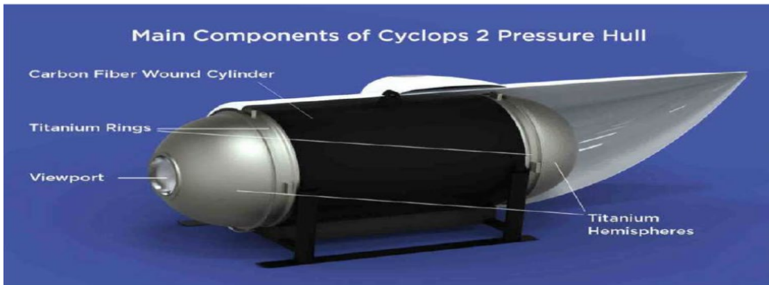
Figure 155: Main components of the CYCLOPS II (TITAN) pressure hull. Source: OceanGate.
