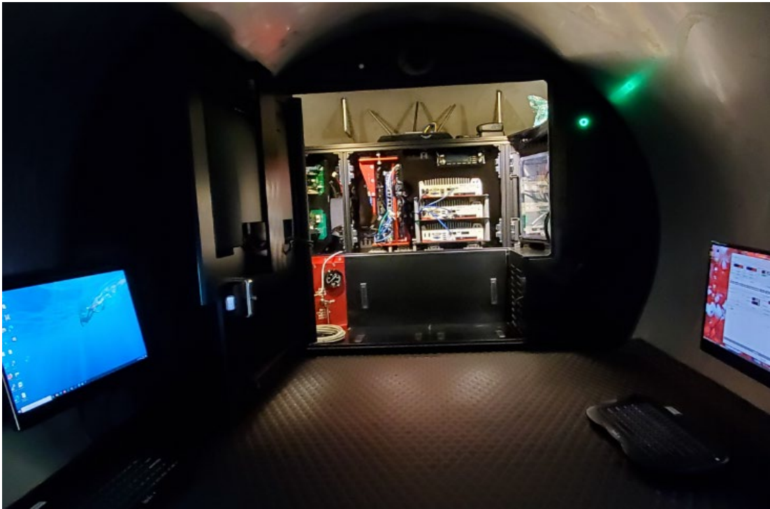
Figure 170: Internal aft compartment of TITAN. The TITAN's three servers are visible within the aft dome. Source: OceanGate.
