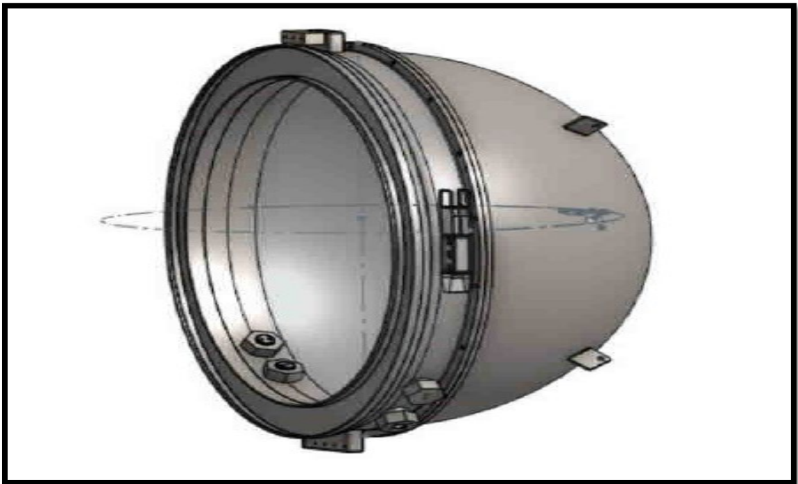
Figure 86: CAD drawing of TITAN's aft dome and segment. Source: OceanGate.
