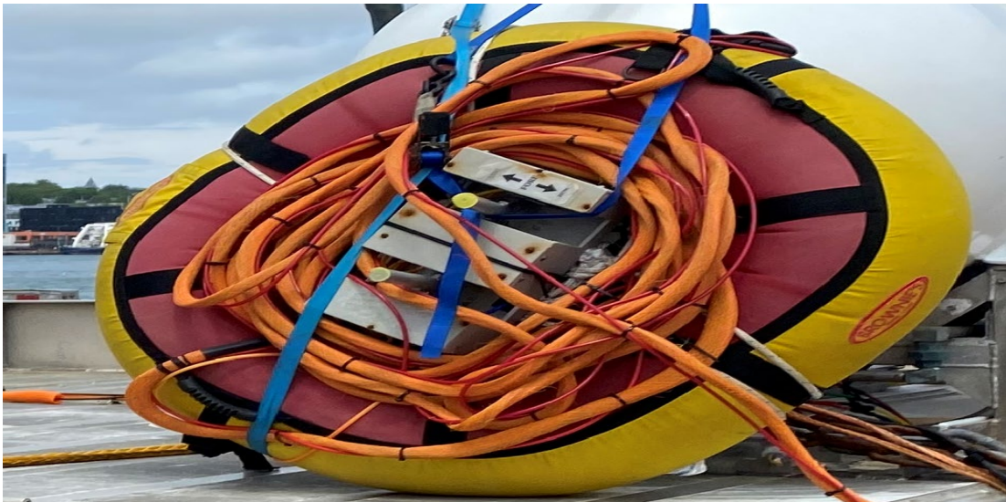
Figure 115: Photo of the air regulator system used to raise the LARS taken by MBI in St. John's, Newfoundland on June 25, 2023. Source: USCG.
