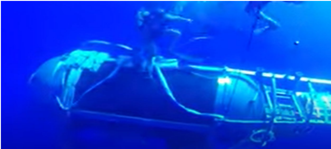
Figure 124: Divers rigging the first TITAN hull for an unmanned dive in 2018. Source: OceanGate Expeditions.
