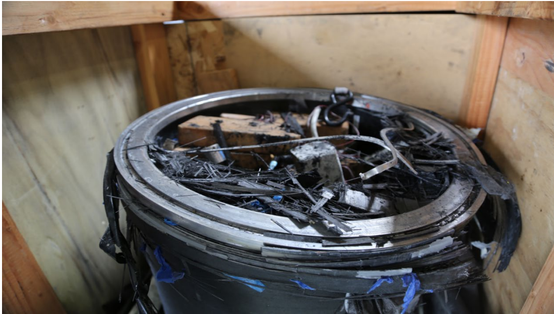
Figure 79: Fourth one-third scale model produced by Spencer Composites post-implosion. Source: OceanGate.
