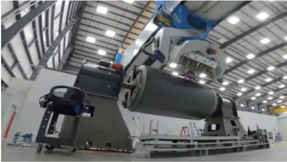
Figure 145: Electroimpact, Inc. AFP machine laying up the final TITAN hull. Source: OceanGate Expeditions.
