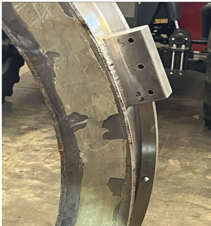
Figure 268: Aft segment with remaining adhesive. Source: USCG.
