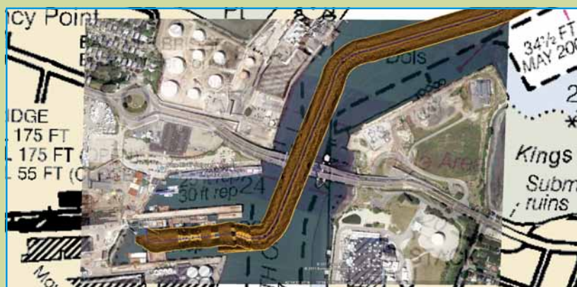
Actual track of an unmanned underwater vehicle (UUV) overlaid on a satellite photo and nautical chart. The UUV transited submerged from Pt. Allerton in Boston Harbor back to its home pier following the normal traffic scheme, surfacing for occasional GPS updates outside the scheme so as not to interfere with surface traffic. Courtesy of Bluefin Robotics.
