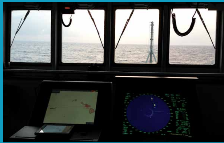
Promoting safe navigation with the electronic chart display and information system includes integrating the visual lookout with radar and ECDIS scanning techniques. Photo courtesy of the author.
