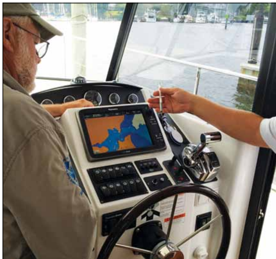
GPS/chartplotters are as common as compasses aboard recreational craft and are increasingly integrated with steering and engine controls. All photos courtesy of Mr. Kevin Falvey.
