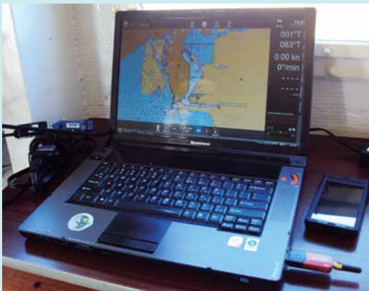
This PPU uses a Bluetooth connection to the pilot plug. All photos courtesy of the American Pilots' Association.
