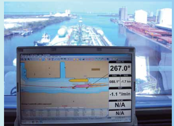
A PPU uses the wide area augmentation system.
