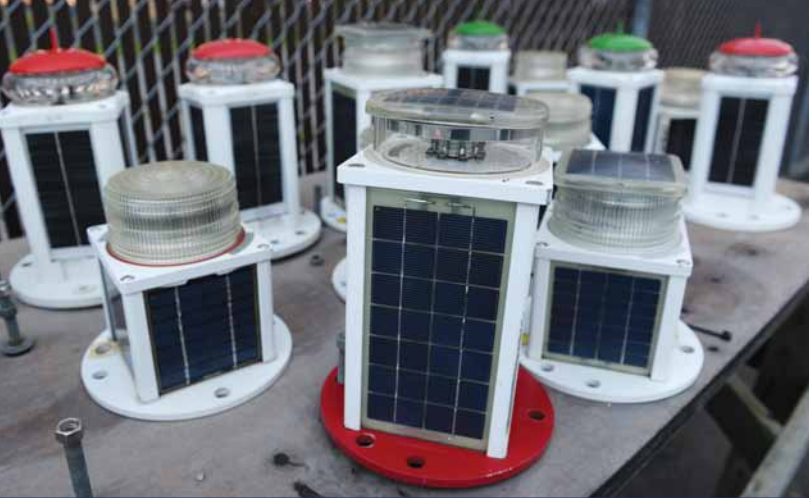
Solar LED lights used on aids to navigation at Coast Guard Station, Crisfield, Maryland. U.S. Coast Guard photo by Petty Officer Lisa Ferdinando.
