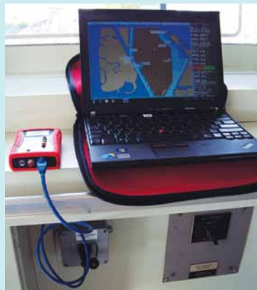
A PPU with Bluetooth connection to an independent differential GPS and AIS pilot plug interface.
