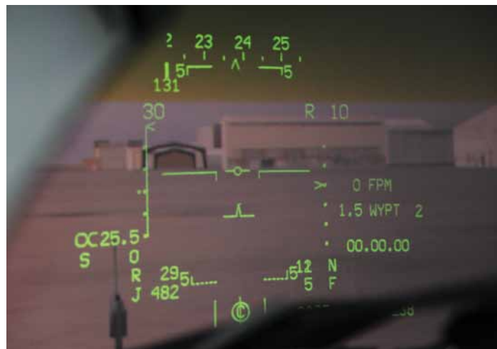
This aviation heads-up display shows many of the aircraft functions including altitude, speed, and level to help pilots keep their eyes on the environment. U.S. Marine Corps photo by Lance Cpl. Cory D. Polom.
