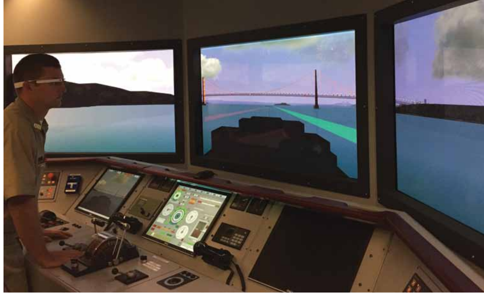
WIAR study tool—Cal Maritime full mission simulator. Photo courtesy of S. Pecota, California Maritime.
