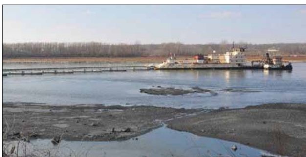
(Right) Dredge Hurley on the Mississippi River at Thebes, Illinois, in February 2013, dredging during extreme low water as part of efforts to keep the navigation channel open for use. Army Corps of Engineers photo by Jim Pogue (Bottom) The Mississippi River Basin. Image by Rainer Lesniewski | Shutterstock.com
