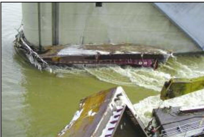
Barges that had broken free from towboat Jon J. Strong were damaged and sank, which obstructed the dam at Belleville lock and dam, mile marker 203, Ohio River. USCG photo by MST1 Kyle Chapman.
